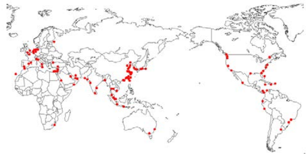
Fig. 1 Locations of Ports Holding Mooring Facilities Dedicated to Containers (Top 100 Ports by Handling Volume)
