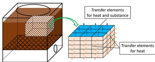
Fig. 10 Mesh of the FEM model
