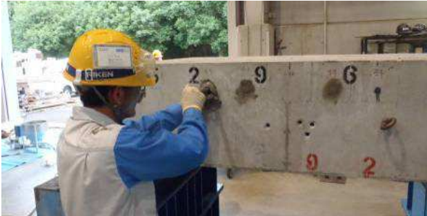
Figure-7 Actual situation (rebar inserting)
