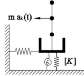
Figure 11: Spring-dashpot of foundation-soil system
