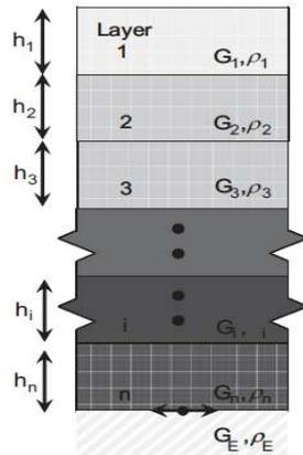
Figure 6: One-dimensional soil deposits model
