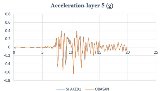
Figure 10: Equivalent-linear response analysis
