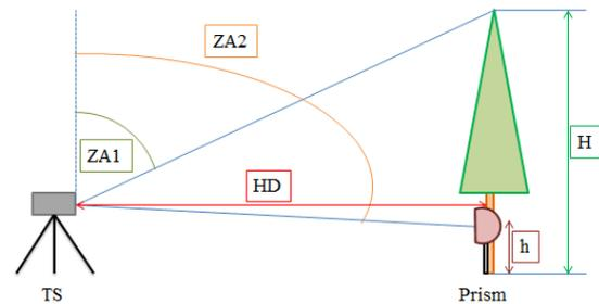
Figure 2.7 Conceptual diagram of the tree height measurement using a TS and a prism
