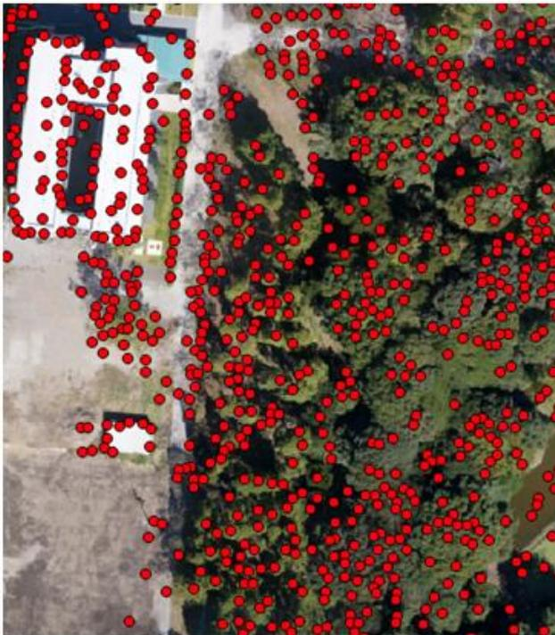
Figure 3.1 Result of the extraction of tree position by LMF method
