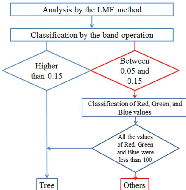
Figure 2.7 Flowchart of discriminating tree by LMF and band operation
