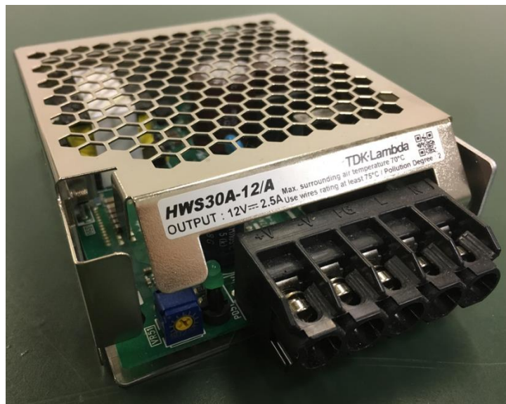
Fig.38 DC Power Source
