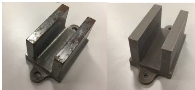
Fig. 16 Electromagnets (core material: SS400 ABS)
