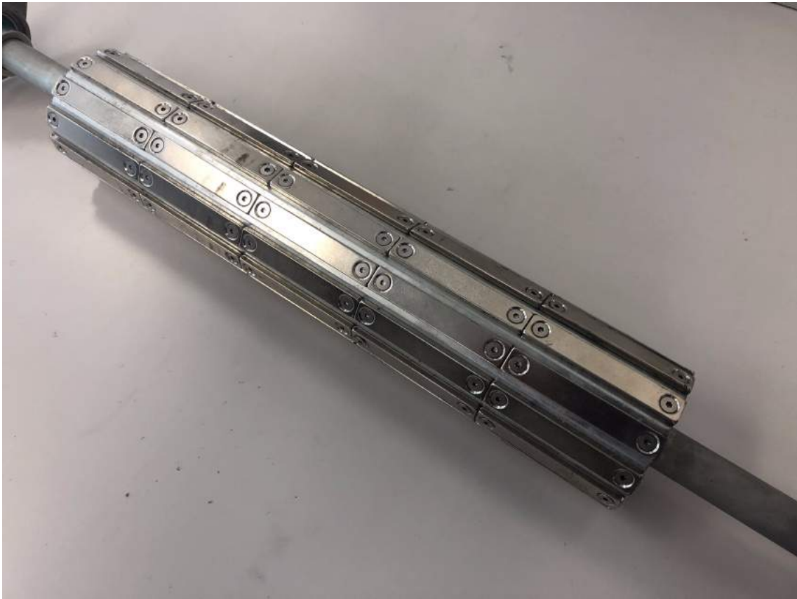
Fig. 9 Rotor with permanent magnet
