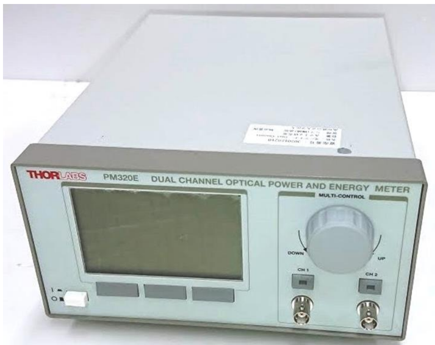
Fig. 4.2.3 THORLABS Dual-channel Benchtop power and Energy Meter Console used for experiments.
