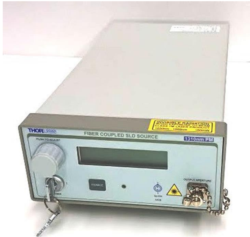
Fig. 4.2.2 THORLABS PM Benchtop SLD source used for experiments.
