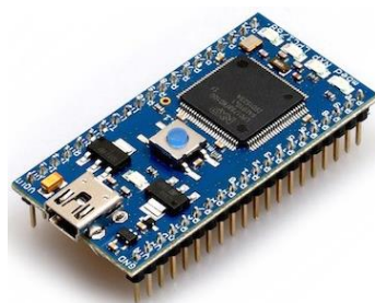
Fig.3.9 Mbed 1768 manufactured by ARM (9)
