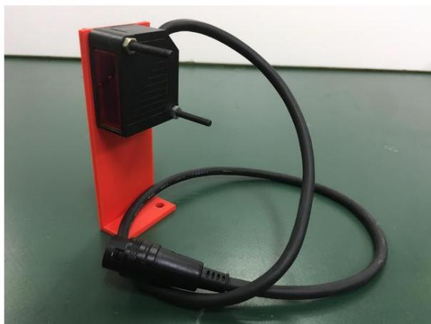
Fig.3.15 Reflective sensor (OMRON)
