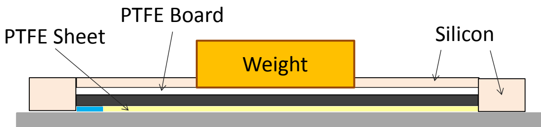
Fig.4-2 Experimental set-up of molding CFRP laminates (The weight is removed during cure process)
