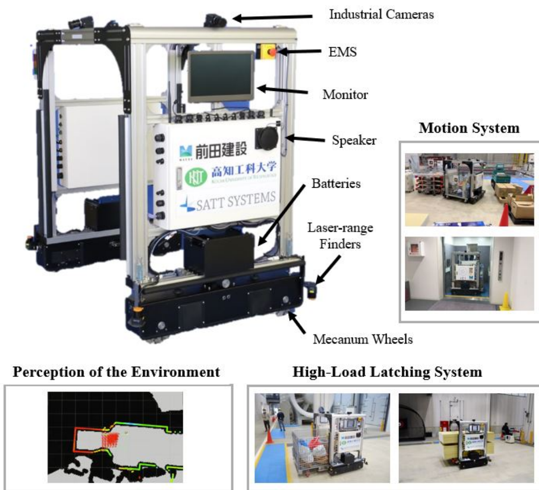
Figure 3-9: A gate-type material handling robot.
