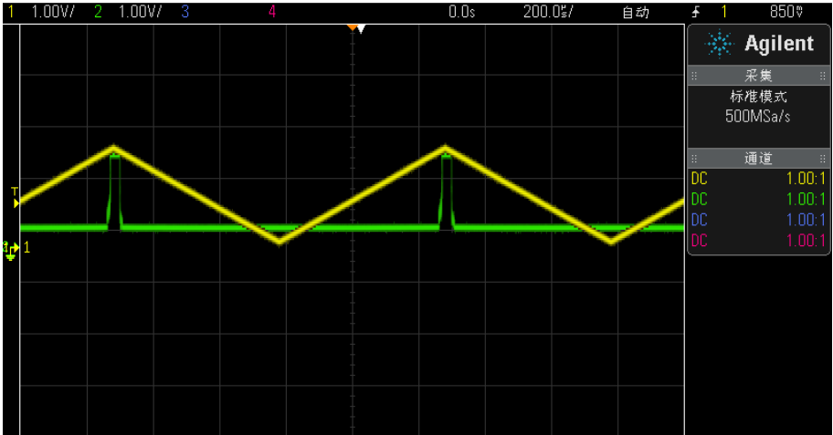
Figure 4.8 The Hysteresis measurement of the proposed window comparator for an input voltage close to the supply voltage.
