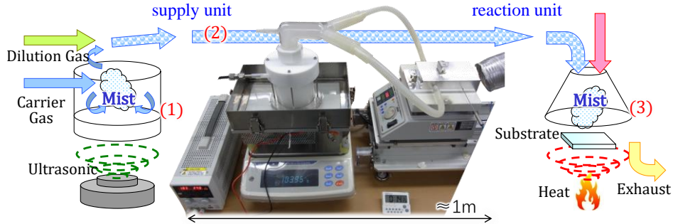
Fig. 2.1 Schematic structure of Mist-CVD system [1]
