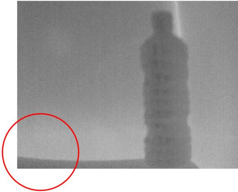
Figure 3-10 Barrel distortion of IR image when range distance exceeds 28 cm
