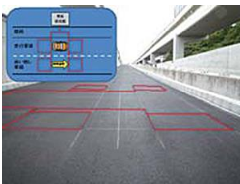
Fig.1-2 Loop coil type vehicle detector (4)
