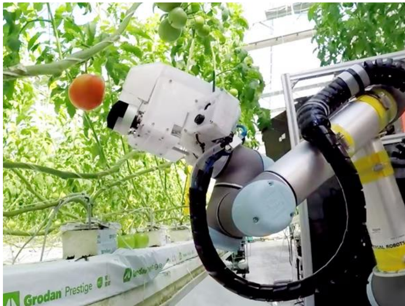
Fig1.3 Vertical articulated manipulator [4]
