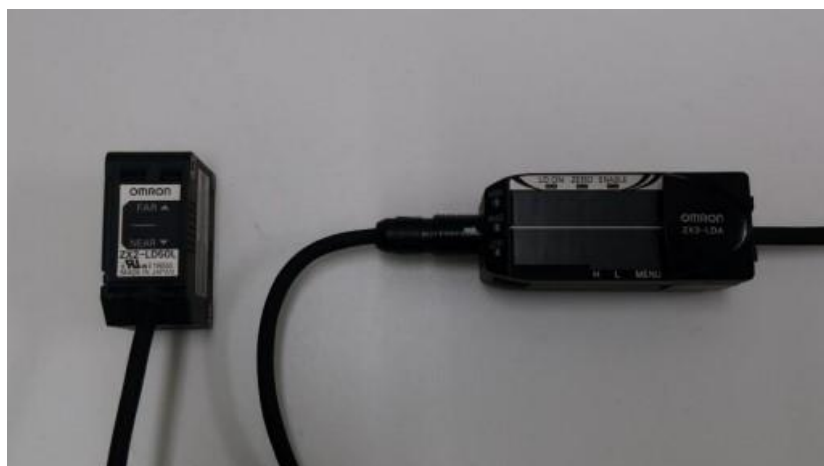
Fig. 38 Laser sensor (OMRON company made ZX2-LD50L), Amplifier(OMRON company made ZX2-LDA)
