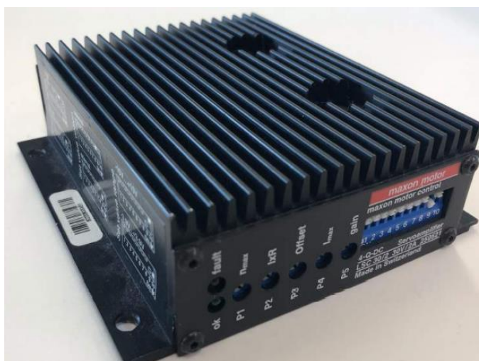
Fig. 35 Servo amplifier (MAXON company made LSC 30/2, 4-Q-DC )
