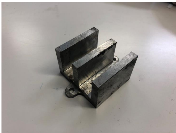
Fig. 8 Electromagnets (core material: SS400)
