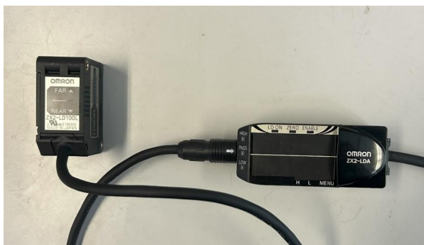
Fig. 39 Laser sensor (OMRON company made ZX2-LD100L), Amplifier(OMRON company made ZX2-LDA)
