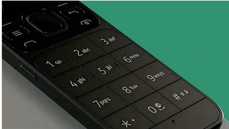
Figure 2.1 A feature phone with a 12-key keyboard. Arrow keys and the backspace key are put above the keyboard.
