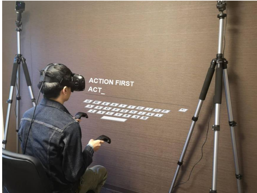
Figure 5.3 A participant in the VR text entry task with handheld controllers and the virtual keyboard floating in the head-mounted display. In this picture, there was an angle of 30 degrees between the virtual keyboard and the ground.
