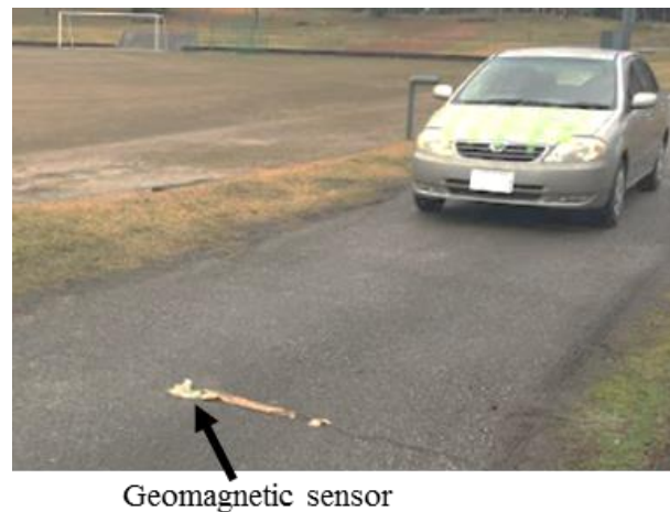
Fig. 2-1 Vehicle runs over a sensor
