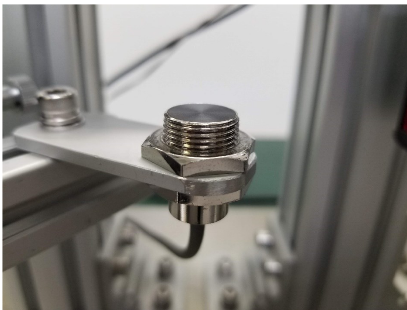
Fig.5-4 Eddy current sensor
