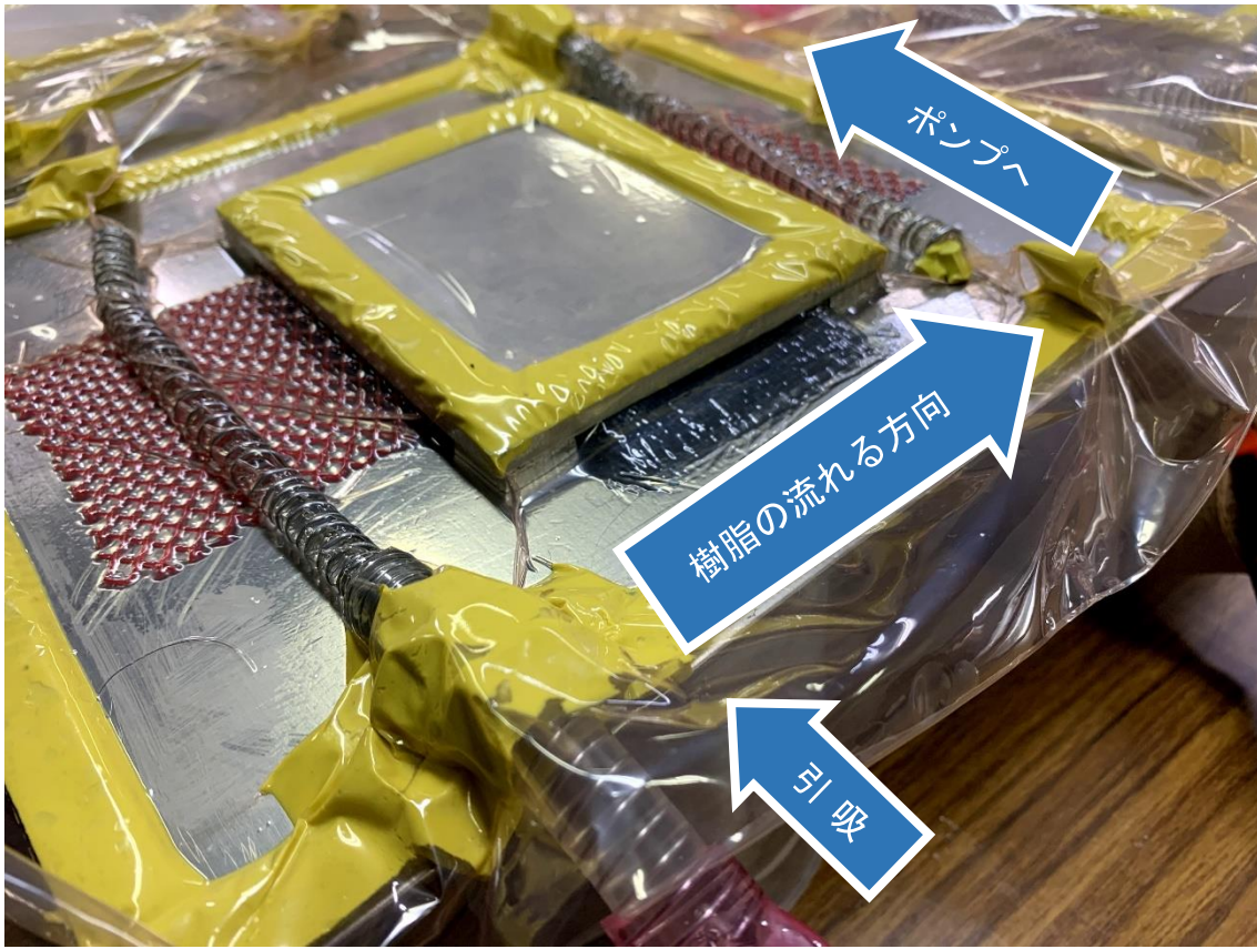
Figure 15. Picture of VaRTM process in this experiment
