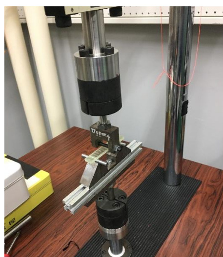
Figure 20. Picture of 3-point bending test
