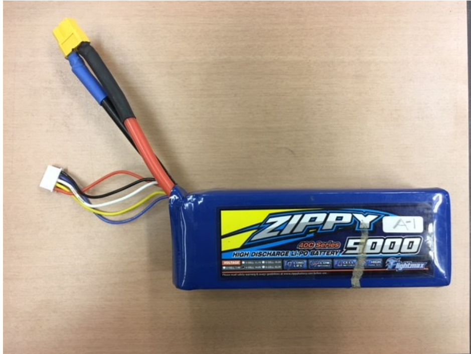
Fig.2-3 battery(ZIPPY5000mAh 4S 40C)
