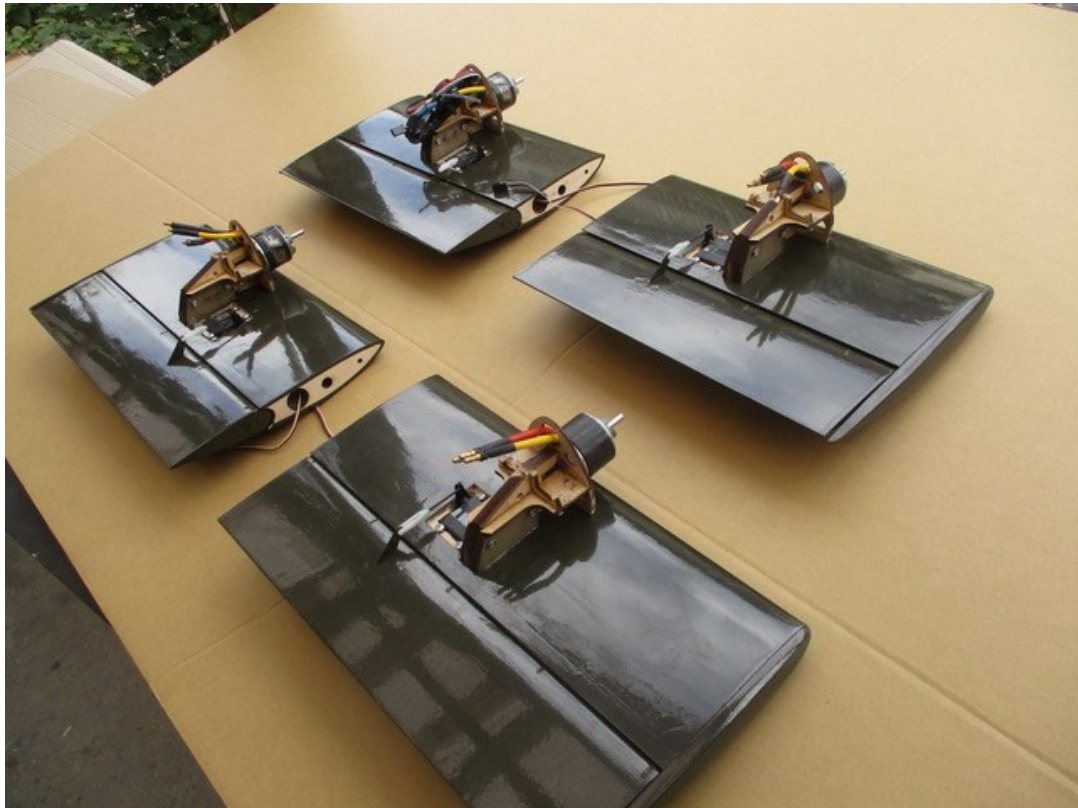
Fig.3-1 wings and motor mounts
