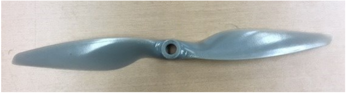
Fig.2-2 propeller(10inch×5.5pitch)
