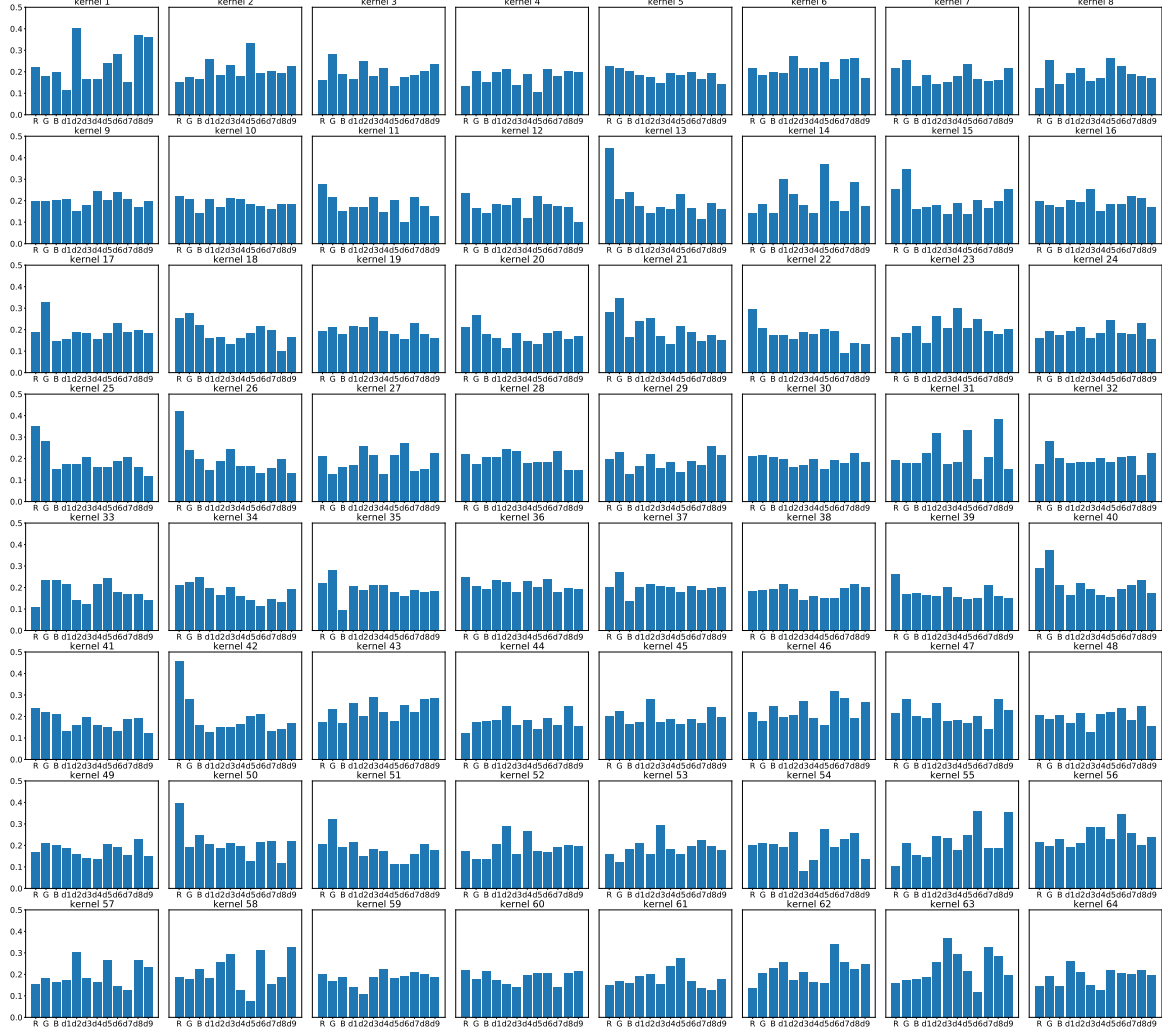
Figure 5.7: The sum of the absolute values of each input channel for each kernel. The horizontal axis represents the different input features of the segmentation module, R, G, B, d1 , d2 , d3 , d4 , d5 , d6 , d7 , d8 , d9 from left to right. The vertical axis of all subfigures are shown in the same range [0, 0.5] . The graph above shows that the color-ratio maps play an essential role, with some kernels showing larger in the color-ratio maps than in the R, G, B feature map.
