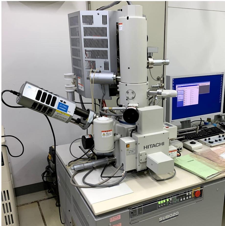
*Fig. 3-4. Field emission electron microscope HITACHI-SU8020*
