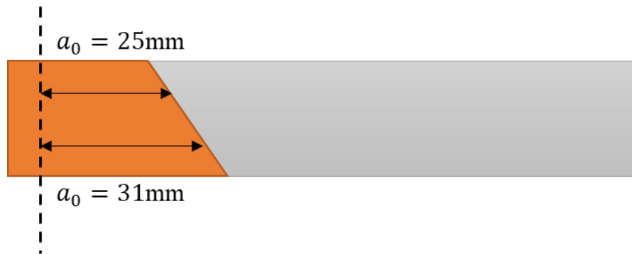
Fig.5.1-4 Dimensions of initial delamination
