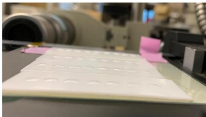
Figure 2. 7 Water droplets on the plasma-treated PTFE in size of 70 mm x 20 mm to examine the homogeneity of plasma treatment.
