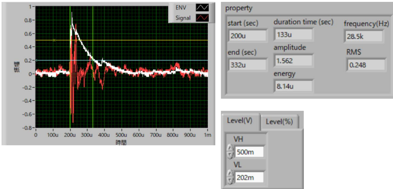
Fig.3.4 Analysis window of AE properties on the application (Threshold levels were set by Volt)
