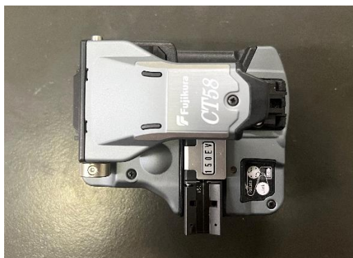
Fig.3.3-4 Optical fiber cutter (for optical fibers with an optical fiber diameter of 0.08)
