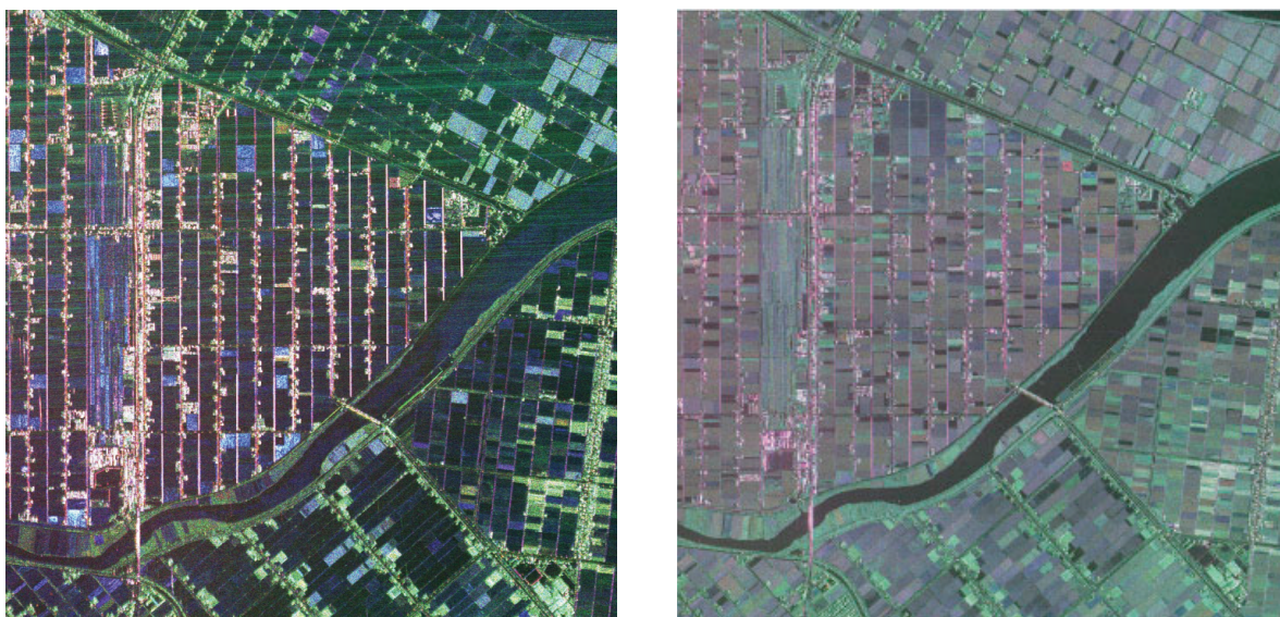
Figure 4.6: Pi-SAR L-band (left) and X-band (right) image of Kojima district, Okayama, Japan. The azimuth direction is from top to bottom and the range direction is from right to left. The image of size approximately 4 km in both directions was acquired on the 13th of July 1999, and the rice plants were almost fully grown with irrigation water underneath.
