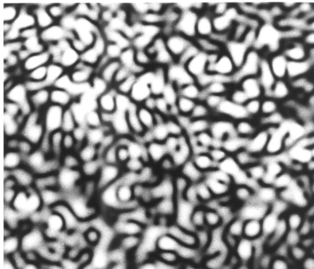
Figure 1.1: Far-field speckle pattern (courtesy of Prof. Kazuo Ouchi, Kochi University of Technology).
