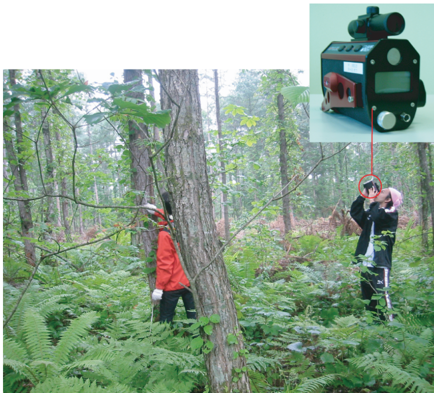
Figure 5.9: Measuring tree height and girth at the breast height. The laser distance measure shown in the right top corner is used to measure tree height.
