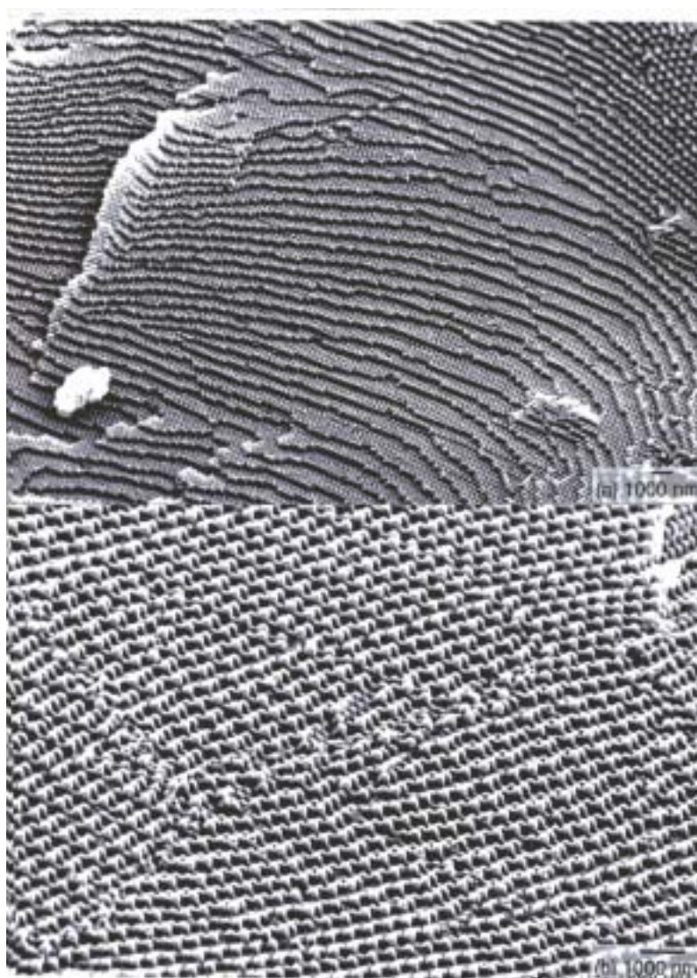
Figure 1-8 (b) Regular arrangement composed of p4VP-microgel and pSt microgel. 20 p4VP/pSt = 1/2 mol/mol, p4VP 260nm, pSt ;190nm.
