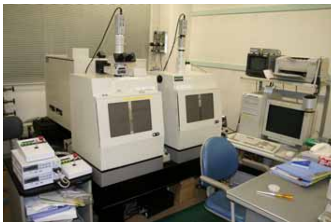
Fig. 5.5. A photo of Raman spectroscopy system (JASCO, NR-1800) used in this research work.
