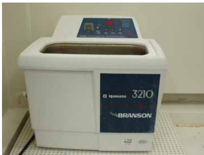
Fig. 2.4. The ultrasonic generator used for cleaning.
