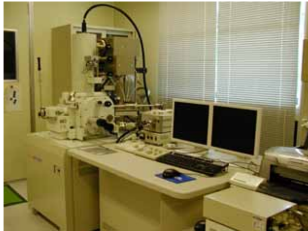
Fig. 5.13. Energy Dispersive X-ray Spectroscopy (EX-23000 BU) combines with a Field Electron Emission Microscope (JEOL JSM-7400).
