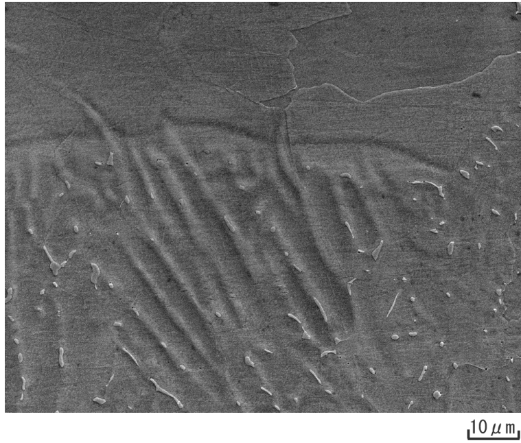
Fig. 2-9 Solidification mode of AF observed in the 16-8-2 weld metal.
