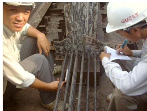
Fig.5.2.5: Measurement of strand elongation
