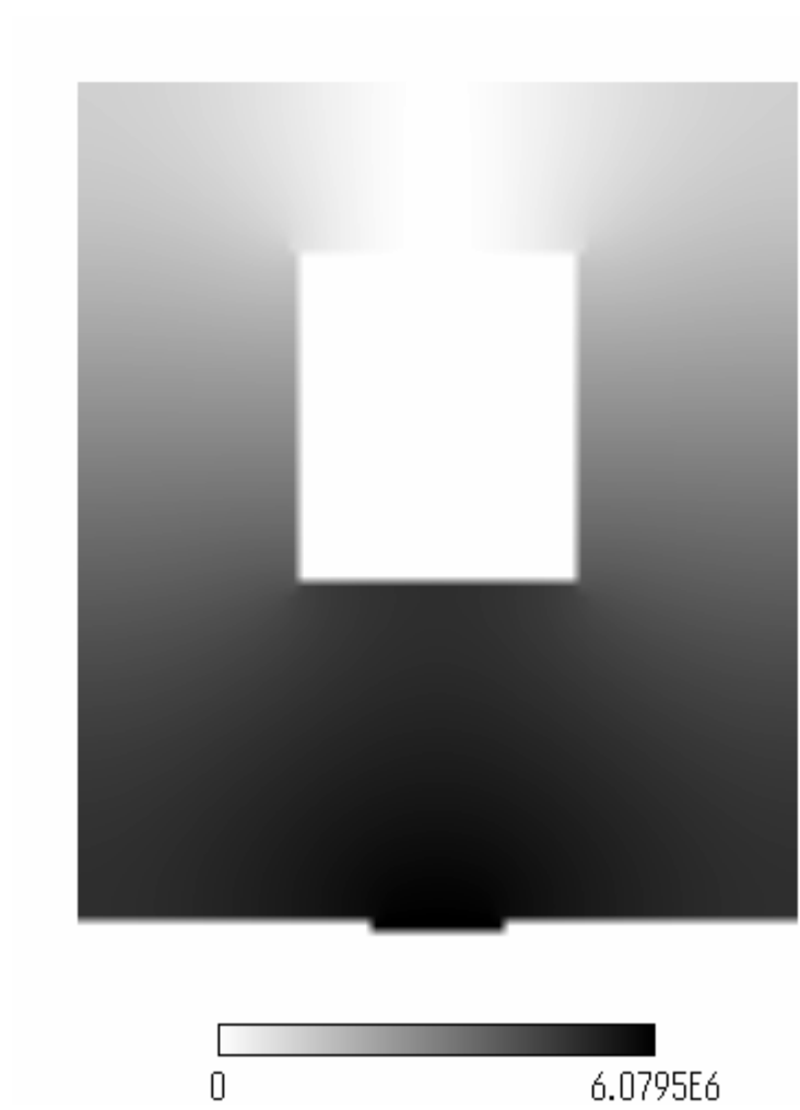
Fig 4-24 Pressure distribution (Pa), when mould temperature=100°C
