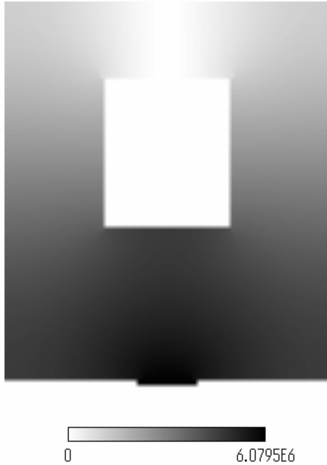
Fig 4-20 Pressure distribution (Pa), when mould temperature=150°C
