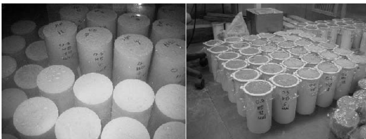
Fig III.3-1: Curing methods: wet curing and seal curing
