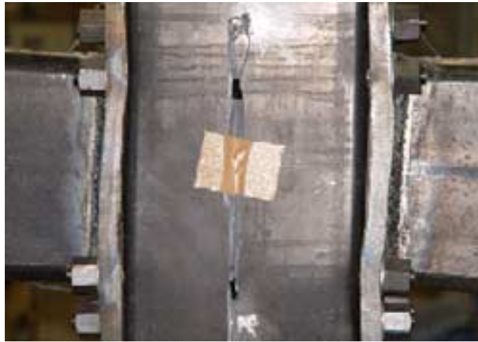
Fig2.16 Deformation of PC bar Flange
