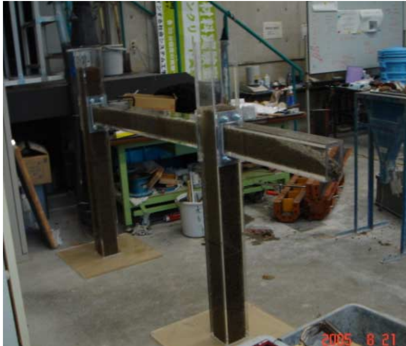
Fig4.3 Typical Test Setup for Concrete Flow Simulation Using Visual Model of Fresh Concrete
