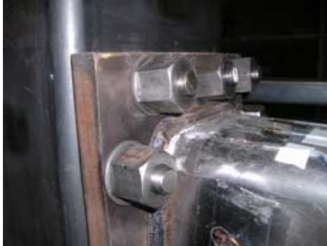
Fig2.14 Weld Fracture in Specimen CPP
