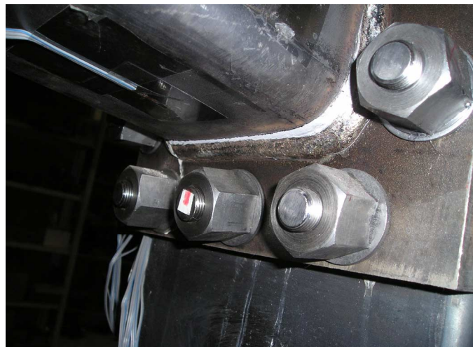
Fig2.15 Weld Fracture in Specimen CPP 1
