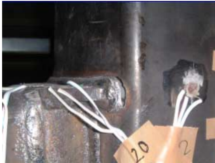
Fig2.11 Weld Fracture in Specimen CDF
