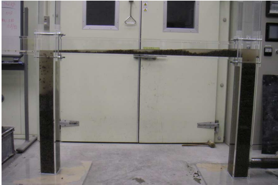
Fig4.8 Situation of the Whole Subassembly after Pouring Concrete in Experiment Project II
