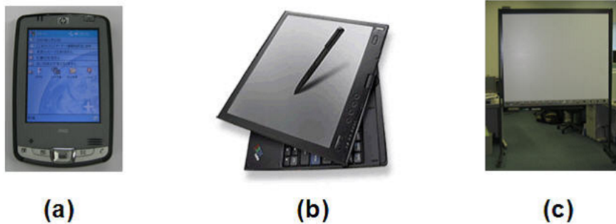
Fig. 1.1 A sample of pen-based devices. (a) small size devices: PDAs; (b) medium size devices: Tablet PCs; (c) big size devices: whiteboards.
