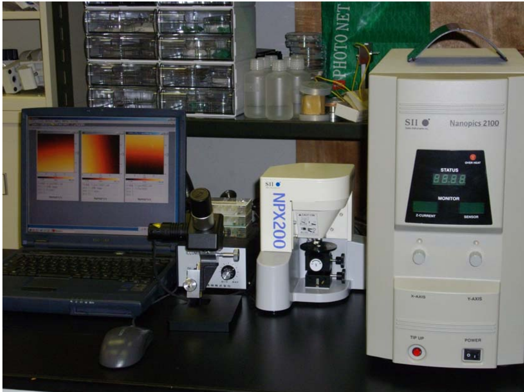
Figure 3.2. SEIKO Nanopics 2100 AFM facility is shown here, installed in the Accelerator lab in the Department of Electronic and Photonic Systems Engineering at KUT.
