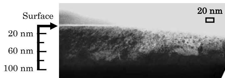
Fig.2 Cross-sectioned TEM micrographs for Fe implanted \text{TiO}_2 with 0.8 \times 10^{17} ions/ \text{cm}^2 .
