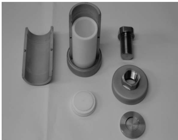
Fig.2-3 Pressure vessel used in synthesis
