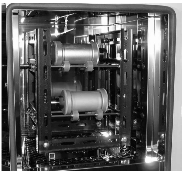
Fig.2-4 Hot drying oven used in hydrothermal synthesis
