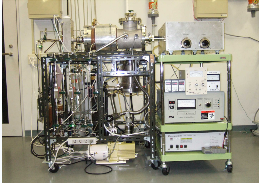
Fig. 2.4 (a) RF-PECVD apparatus used for DLC deposition.
