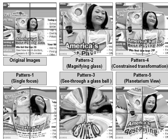
図 6.4 注視域の拡大パターン (Pattern-1:Single focus, Pattern-2:Magnifying glass, Pattern-3:Seeing through a glass ball, Pattern-4:Constrained transformation, Pattern-5:Planetarium view)
