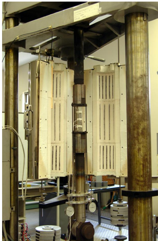
Fig. 2-9. 50t heavy-loading creep testing machine used for testing the specimens of the thick welded joint.
