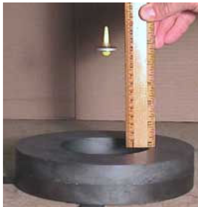
Fig.1.14 A photograph of a flux path control suspension mechanism.
