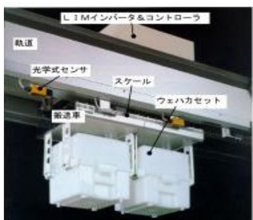
Fig.2.1 A hanging type transmission vehicle of Toshiba using electromagnets
