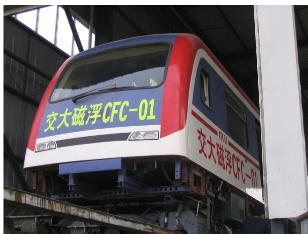
Fig.1.17 The high-temperature superconducting maglev CFC-01 in China
