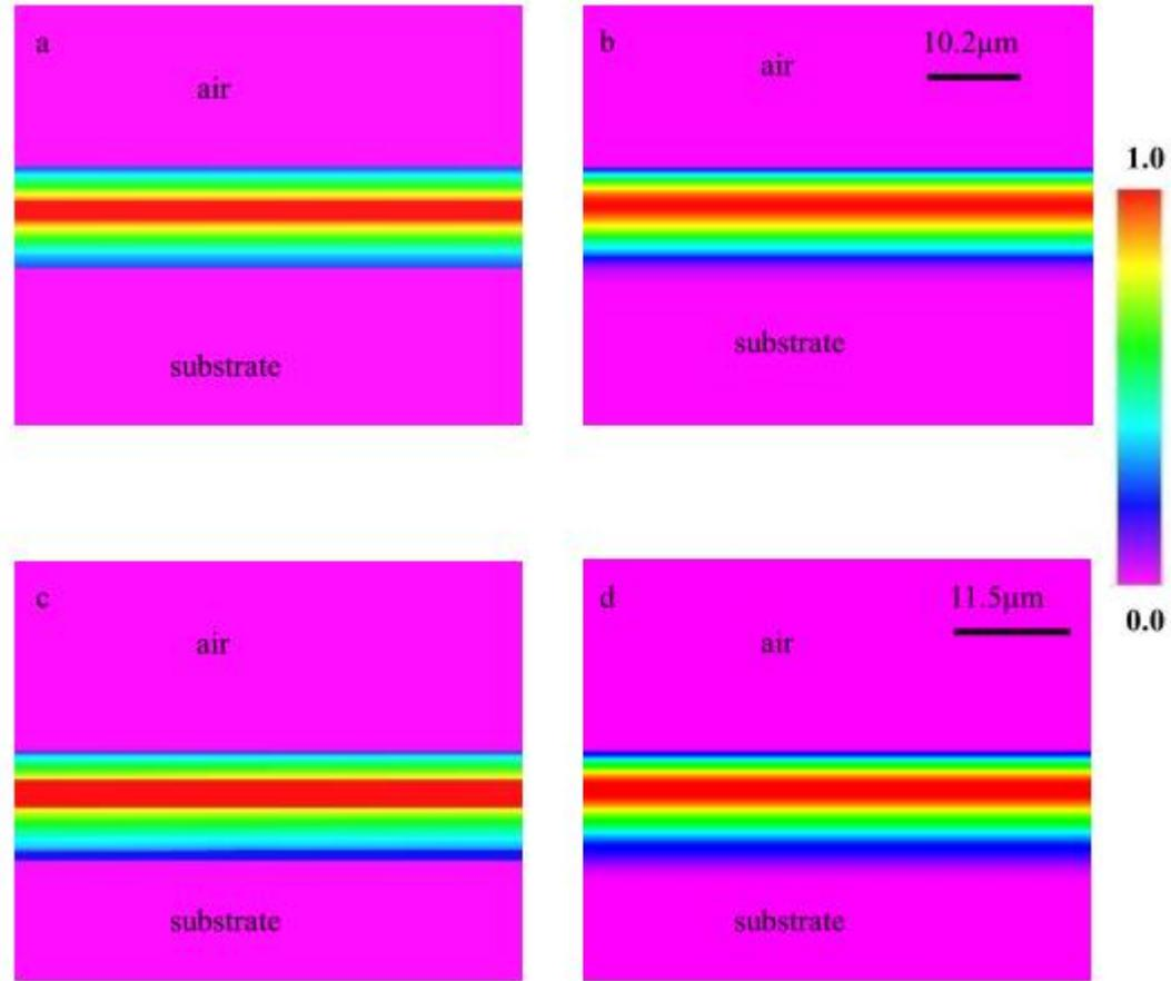
Fig. 5.1.3 Near-field intensity distribution experimental result (a)GLS and (c)GLSO; simulation using BPM (b)GLS and (d)GLSO
