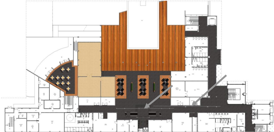
Figure 2.8. Examples of errors due to the incorrect determination of bench marks by contractor, so that the "as line" of column shifted during construction process, which results in some columns stand in the middle of the building aisle (Source: RFD Studio Consultant).
