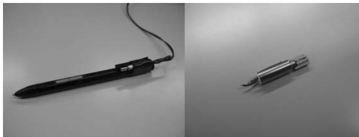
Fig. 2.1 Stylus with an attached motor and the motor.
