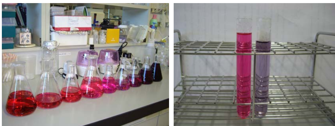
Fig.3.6. Red pigment fractions obtained from ODS open column chromatography separation and the comparison of the first and the last eluted fractions of the pigment.
