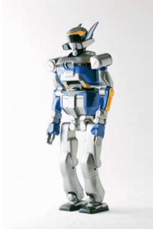
Fig.1.8 AIST etc. HRP series “HRP-2”
